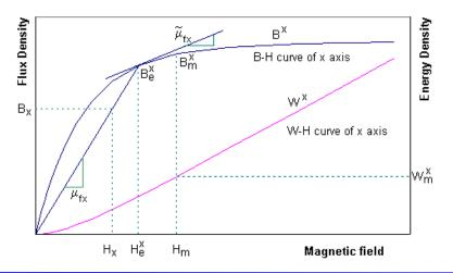
Example (Magnetostatic) - Anisotropic Material
