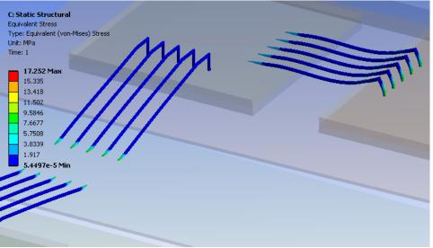
Maximum stress resulting in wires can be compared with the material properties to predict the failure region.
