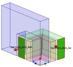
Note: The current value of Coil\_In was 100A and Coil\_Out was 50A in full model. The sectional area of the coil is 1/2 in 1/8 models because it is divided by XY plane. Therefore, the current value becomes 1/2, too.
