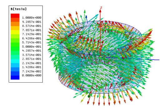
Check the Plots of Brad that we created in last exercise. The difference in the results can be seen. The strength of magnetic filed in radial direction varies with Phi. The function results in for pole magnet as expected.
