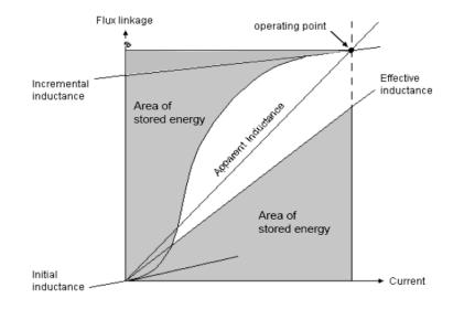
Incremental inductance can also be obtained using Maxwell by setting the parameter *Maxwell 3D > Design Settings > Matrix Computation* to the value Incremental
