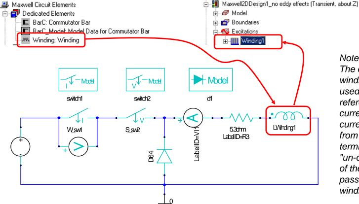
After circuit editor opens, add elements to construct the circuit. Note that the name of the 2. Winding in the circuit (Winding1) must match the name of the Winding in Maxwell (Winding1)
