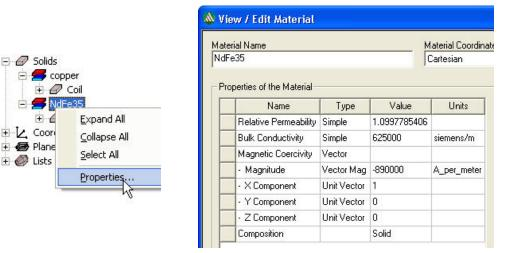
In Maxwell All materials are magnetized in X Direction. Users can change the AL direction as needed
