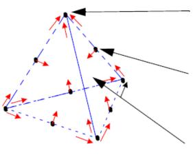
The Components of a Field that are tangential to the edges of an element are explicitly stored at the vertices.
