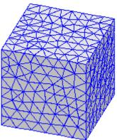
Initial mesh with Length-Based Inside & On Selection set to 20% 9042 elements
