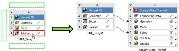
Note: By Dropping Steady State Thermal Analysis System onto Solution tab of Maxwell System we are establishing a link between Solution tab of Maxwell and Setup tab of Steady State thermal Analysis System. This will enable the data transfer from Maxwell to ANSYS Mechanical
