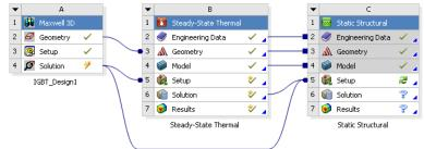
Note: By dropping Solution tab of Maxwell onto Setup tab of Static Structural System, a link will be created between them. This will ensure transfer of Lorentz Forces from Maxwell to ANSYS Mechanical
