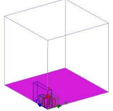
Note: The surface of boundary area (region) is analyzed as a natural boundary condition (Flux is the horizontal compared with respect). Because Flux becomes the horizontal for the YZ plane and the XZ plane in this model, the Symmetry boundaries is not necessary.
