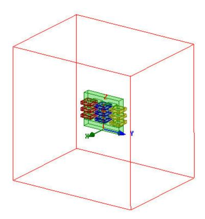
Example (Magnetostatic) - Inductance Calculation
