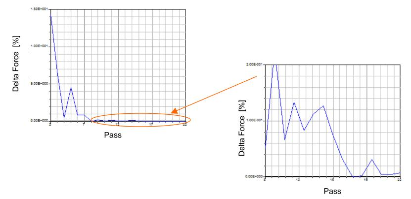
% Change in the Force on the magnet can be used to determine a more effective stopping criteria since this value can be tied directly to the acceptable numerical tolerance on a <u>physical</u> variable
