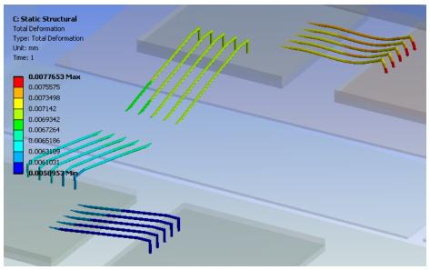
Note: Deformation images are magnified. To view results to the scale Change the Result to True Scale
