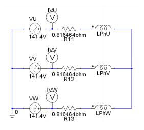
Circuit model of 3 Phase Y connection
