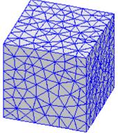
Initial mesh with Length-Based Inside-Selection set to 20% 6698 elements
