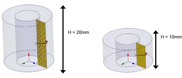
Modeling the Full Coil: Conductor Number = 150 Symmetry Multiplier = 1 Cut the Full Coil in half and use an Odd Symmetry Boundary: Conductor Number = 75
