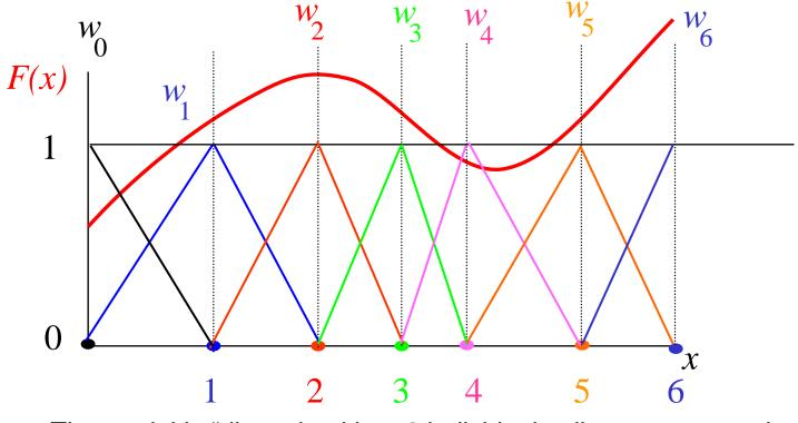
• The model is "discretized into 6 individual cells.  $w_0 - w_6$  are the piecewise linear "basis functions" from which the approximate solution will be built.
