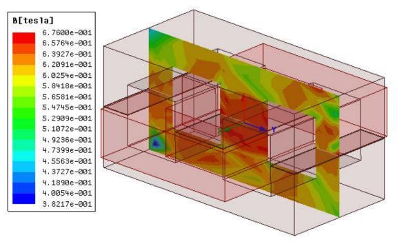
Note: This field plot is for the nominal design case with gap = 0.1mm and ampturns = 100A.
