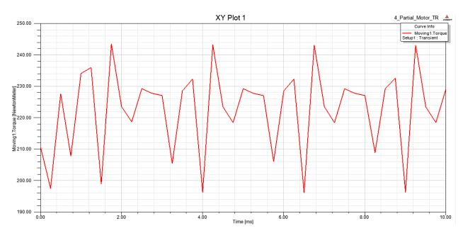
We can see that there are a lot of ripples. The ratio between the torque and the torque ripples is almost 5 percent. This is due to the unique structure of the IPM motor (Internal Permanent Magnets). To limit the ripple, some manufacturers modify slightly the rotor shape around the magnets or add a second layer of internal magnets
