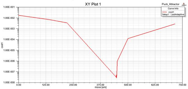
From the plot, it can be seen that minimum value of cost is obtained at around 445 um
