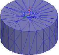
The default is sufficient for many applications in which the curved geometry is not AL itself highly critical to the simulation result, yet where more faceting would result in an unnecessary large initial mesh. Special cases might need added meshing operations to achieve better results.
