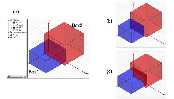
Note: Either Select Clone tool objects before subtracting while subtracting or Duplicate the object (Select the tool object, then *Edit > Duplicate > Around Axis* with an Angle of 0 and a Total number of 2, or use Ctrl+C, Ctrl+V if you are in the original object's coordinate system) before subtracting to retain both objects after the subtraction is performed.
