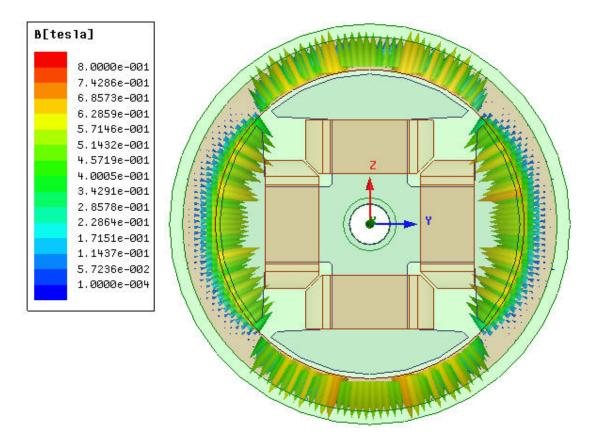
Note: Please note that if the RingMagnet is not set up as anisotropic one (i.e. uniform Nonlinear one) the B field between two magnetic poles will be very large in the theta directions, which will be not as good as user wanted.
