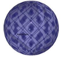
Note: This assigns a radiation boundary to the outside of the sphere, allowing the waves to propagate outside of the sphere. If no radiation boundary is assigned, the interactions of the components may be correct, but the fields near the boundaries will certainly be incorrect. The Poynting vector on the outer surface is a clear indicator of this, which we will explore later.
