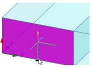
X-axis of the newly created face CS is now aligned with the direction of magnetization of Magnet1
