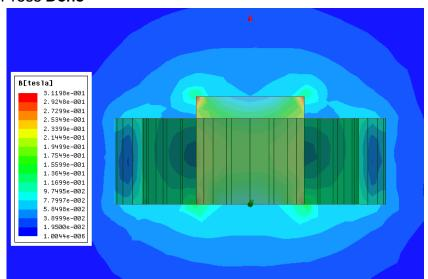
The results show about 0.2 Tesla field in the Center of the Slug which is well within the linear region of the BH curve for most steels
