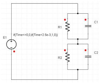
Since the material and geometry information of the two dielectric layers are known, the resistances and capacitances can be calculated with the equations:
