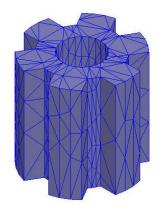
Note : This is initial mesh created by Maxwell. Apart from transient solver, for all other solvers this mesh will be refined for each pass in order to increase accuracy of solution. For Transient solutions, mesh refinement is not done. So it is required to apply appropriate mesh sizes which will be discussed in next few slides.
