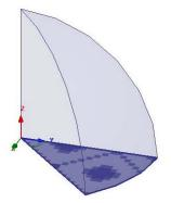
Note: Only one symmetry boundary is required even though three surfaces define distinct symmetries. The two surfaces perpendicular to the ring have a symmetry that is accounted for by the default boundary condition of Zero Tangential H Field - i.e. this is a special case of symmetry, where the symmetric tangential fields are zero. The surface that lies in the plane of the ring has a Flux Normal symmetry, so we need to define this separately.
