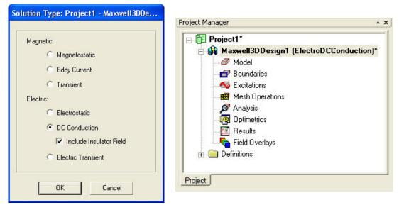
The setup for a ElectroDCConduction simulation is the same as if setting up a DC Conduction simulation in the conducting objects, and setting up an Electrostatic simulation in the insulators. All boundary conditions and excitations for both setups are available when both options are selected. It is up to the user to set up the simulation appropriately in each domain.
