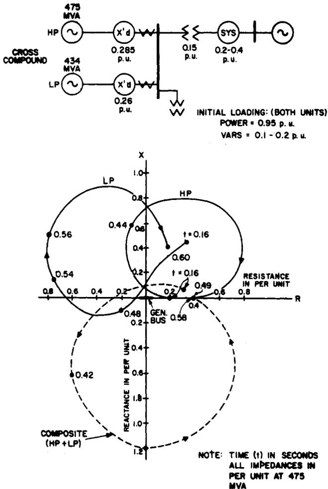
Fig. 4 Loss of Synchronism Characteristic - Cross Compound Unit
