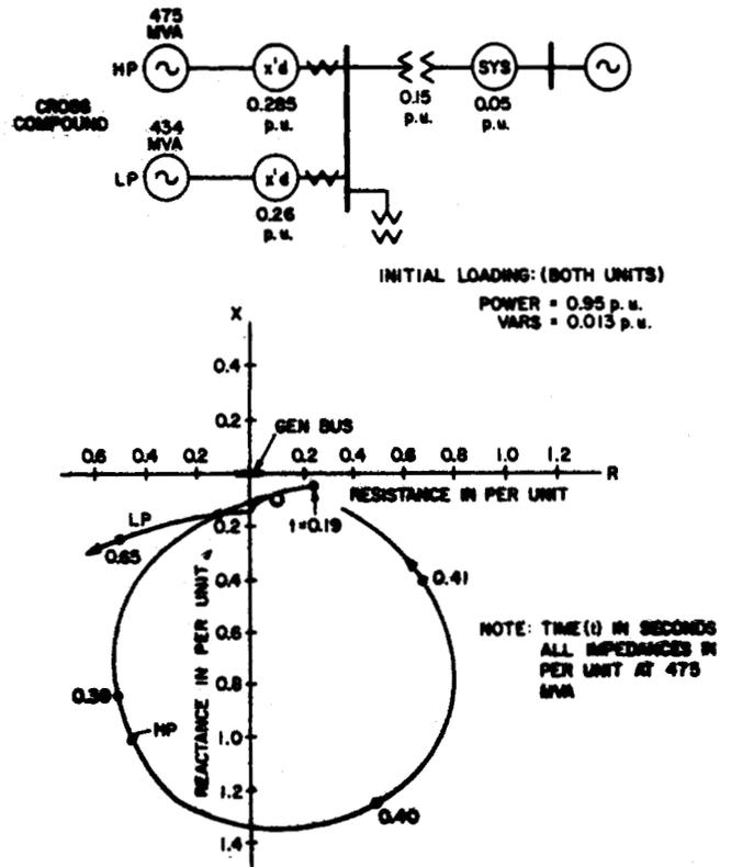
Fig. 3 Loss of Synchronism Characteristic - Cross Compound Unit
