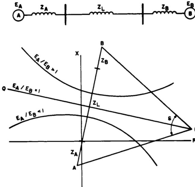
Fig. 1 Typical Out-of-Step Impedance Loci Using Simplified Graphical Procedures
