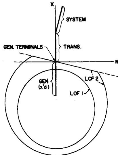
Fig. 5 Typical Loss-of-Field Relay Characteristic
