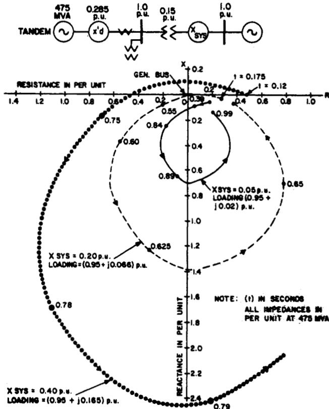
Fig. 2 Loss of Synchronism Characteristic - Tandem Unit
